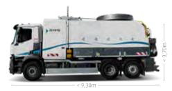
The 3 tanks design of the *ZEPHYR* combination unit allows to realize different kind of interventions on a same tour (septic tanks, municipal networks and grease traps).
